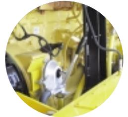
Manual pump for cooler filling on C255-24
