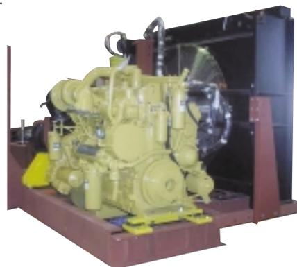
A compact Rig Mount configuration for builders of water well drilling rigs. The 2 stage air end can be provided with Caterpillar engine and side mounted cooler matrix to produce the same air outputs in a base mounted form measuring only 2.25m. x 5.91m. x 2.34m high. This is achieved by a cooler fan driven hydraulically from an engine Power Take Off rather than an in-line cooler arrangement with fan driven by engine shaft.
